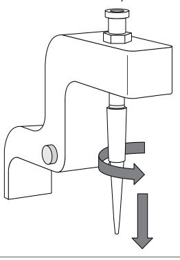
**IMPORTANT!** Improper removal of tips can loosen the metal tip adapter fitting on the Tip Arm and affect instrument operation.
